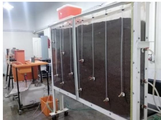
Fig. 1. Experimental model for contaminant transport in porous media
