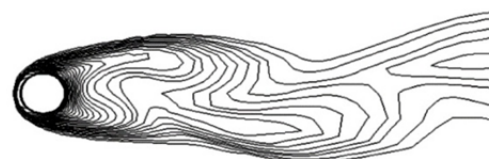
Fig. 21 Instantaneous temperature contour at Re = 150
